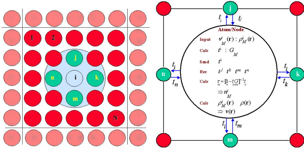
Figure 2: *Left* Schematic of a parallel SCF algorithm. We envision a basic unit cell consisting of  $N$ -atoms labeled  $1, \dots, N$  which is periodically reproduced as indicated. About each atom, for example the  $i^{th}$ , we define a local interaction zone consisting of  $M$ -atoms including itself, for example labeled  $i, j, k, l, m$ . *Right* Schematic of the implementation LSMS algorithm on a massively parallel computer.
